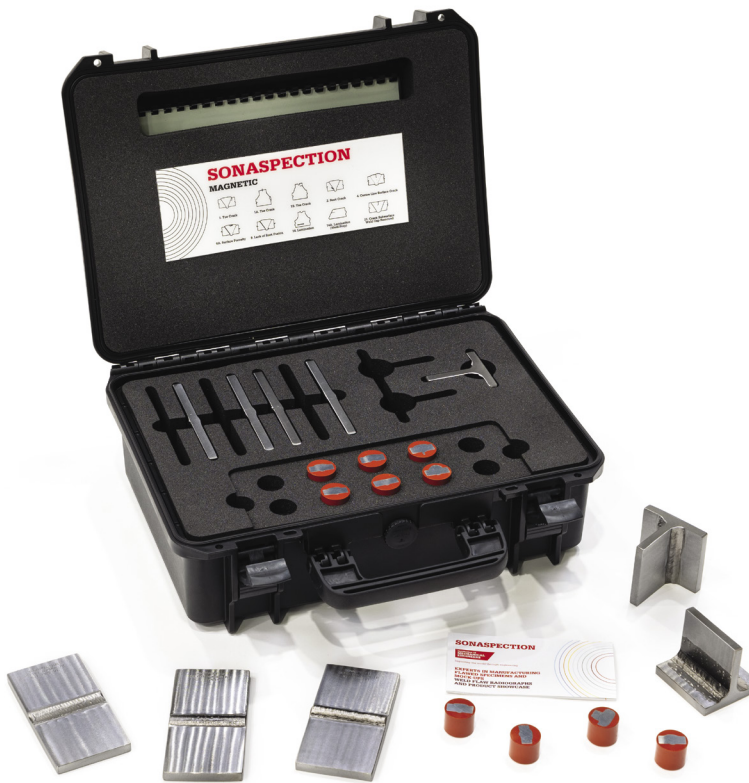
A magnetic particle kit containing 10 macro sections of various flaws
