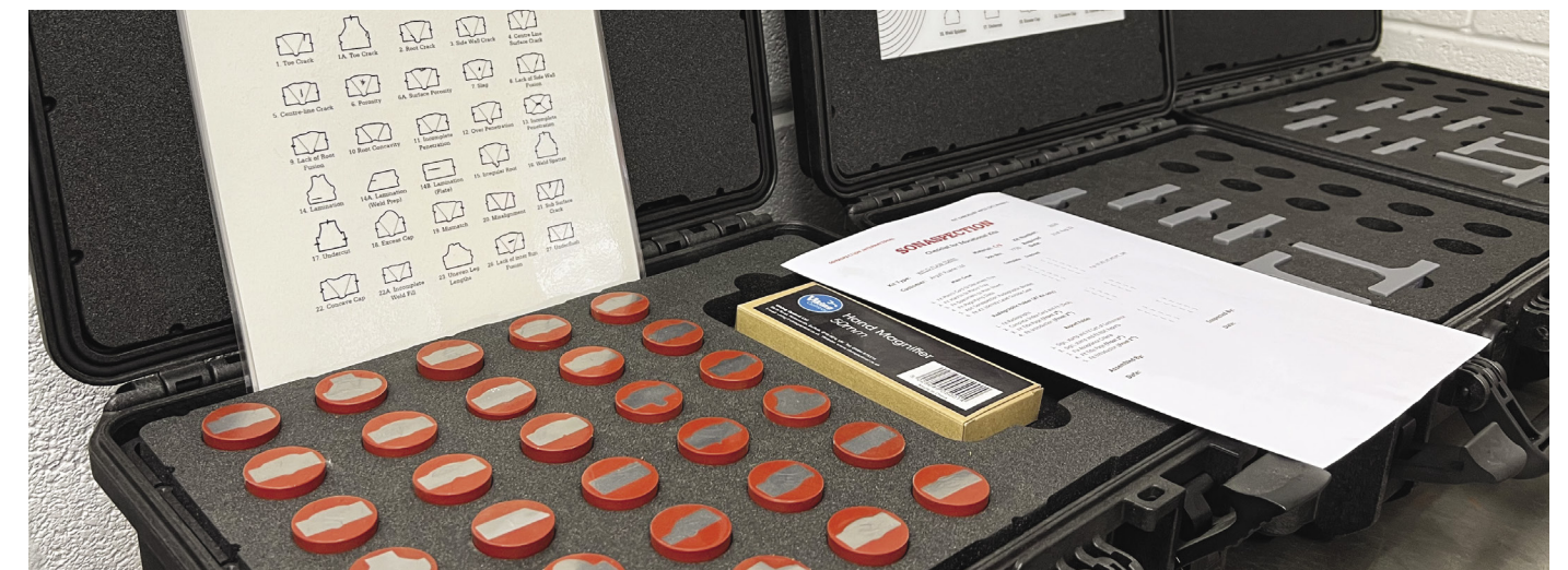
An example of a weld flaw identification kit and 3D printed resin visual testing kit
