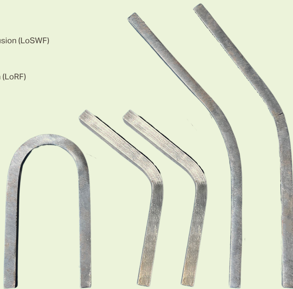
A selection of bend test bar specimens
