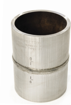
An example of a penetrant testing pipe specimen
