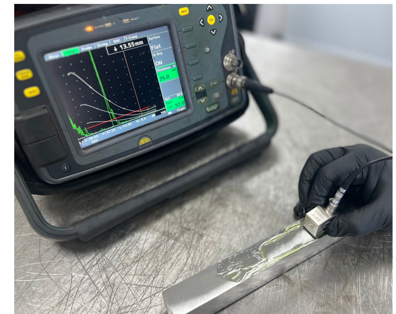
An example of a crack sizing bar
