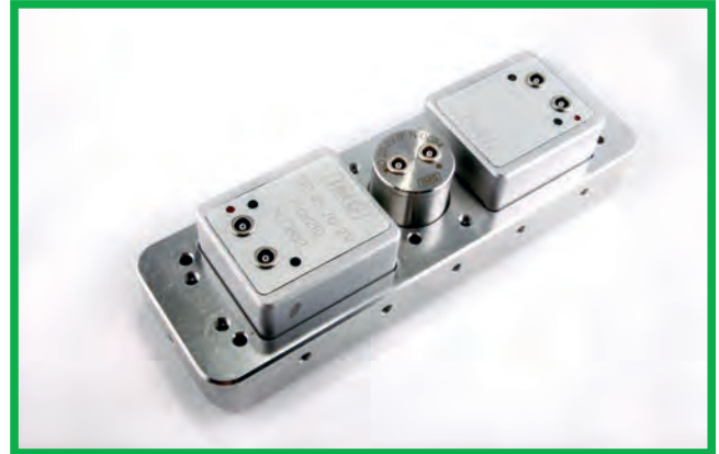
SHOE FOR RAIL INSPECTION with 70° focused twin crystal angled beam probes and one 0° focused twin crystal probe.
