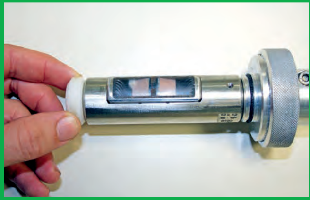
MANUAL BOREPROBE for railways axles inspection with two 45° angled probes and water inlet directly under the probe. Cable length 2 meters.
