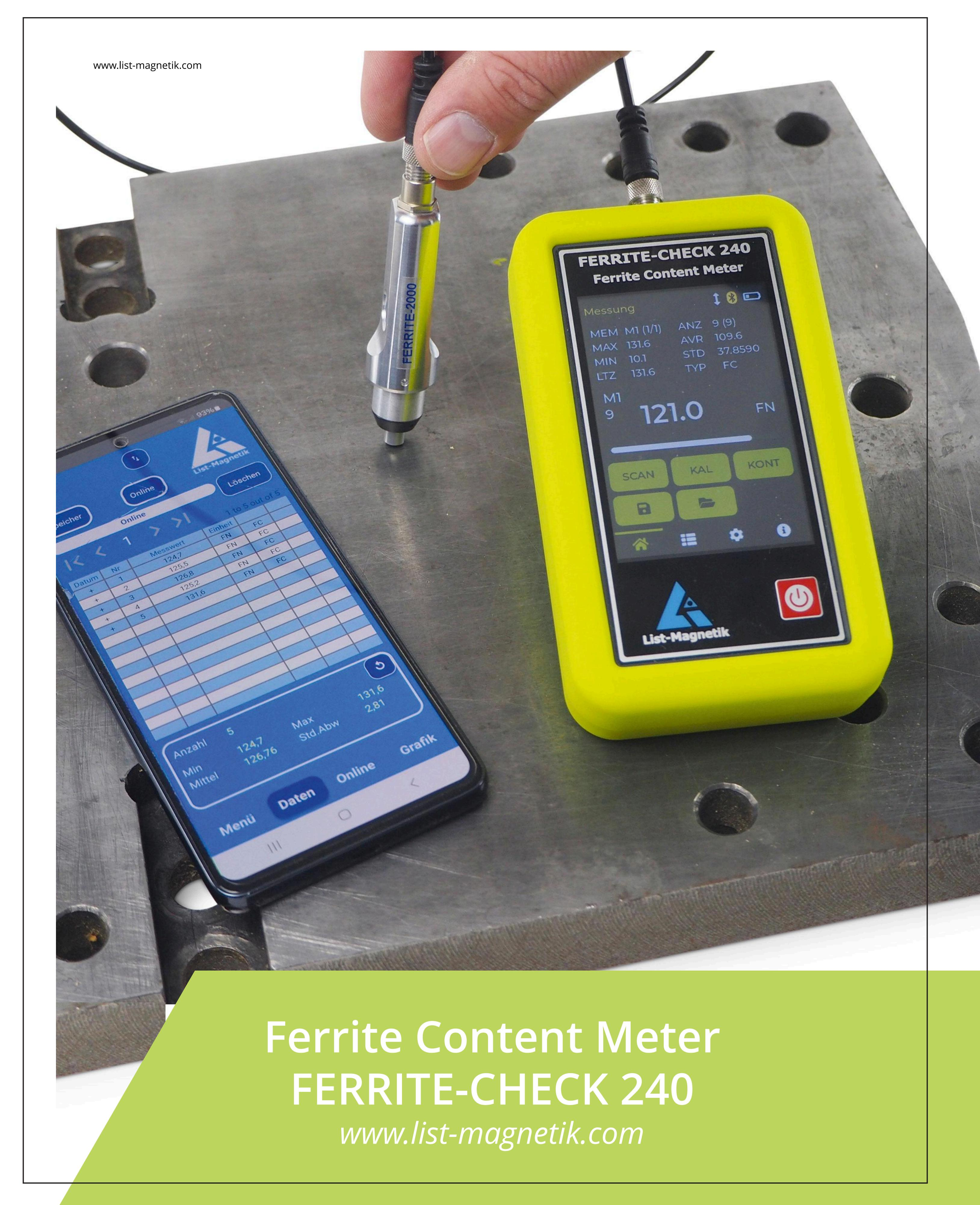
The ferrite content meter **List-Magnetik FERRITE-CHECK 240** is an easy-to-use instrument with color display and external probe for measuring the ferrite content in austenitic and duplex steels according to the Basel standard DIN EN ISO 8249 using the magnetic induction method.
